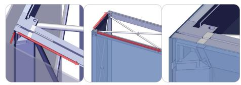
To apply the silicone edge graphic, start by pressing the SEG into the top left corner hub of the frame. Continue to press the SEG into the extrusion bar fabric channel. Keep pressing the SEG into the bar fabric channel until you make down to the bottom right corner hub of the frame. This also works for the second printed graphic option on the back side of the frame when horizontal channel bars are installed.
