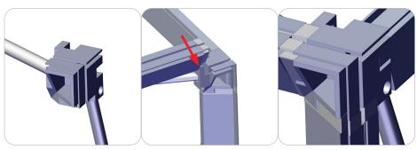
The scissor frames will have this corner hub installed on all four corners, front and back of the frame. This corner hub takes the end caps of the channel bars. The end caps of the channel bar will snap into place.
