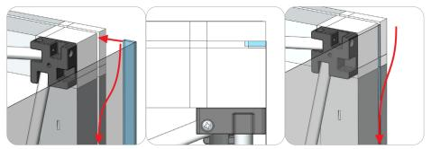
The front printed graphic will also have end cap graphics with silicone edge. Pull the end cap silicone edge to the top of the back corner hub. Start to press in the SEG into the hub and work your way down the side channel. Do the same for the opposite end cap.
