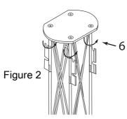
**Step 1.** Unfold Base (A) and expand eachTruss section (B & D). Assemble in order shown, steps 1-6. Figure 1.
